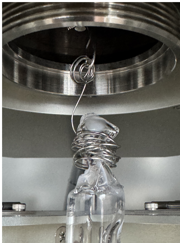
Figure 7: Ampule attachment to the hook with nichrome wire.
